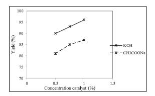
Fig. 4. Effect of base lewis catalyst on biodiesel yield on 300 W microwave power
